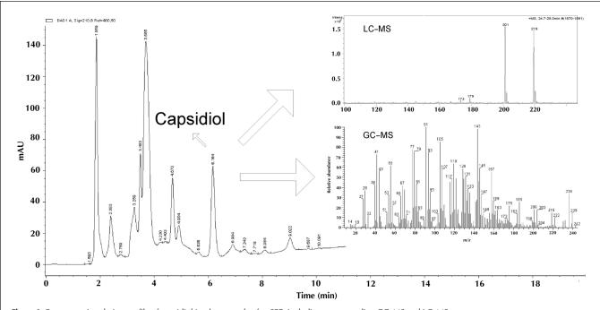
Figure 2. Representative elution profile of capsidiol in plant sample after SPE, including corresponding GC-MS and LC-MS spectra.
